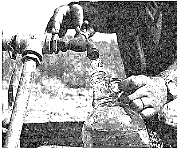
Sampling renovated sewage water pumped from 30-ft depth in the center of the Flushing Meadows Project.
